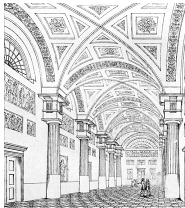
The Column as free-standing sculpture has lost its framing entablature to a ballooning vault - in the 1822-27 design for Court of Requests in the proposed House of Lords.
